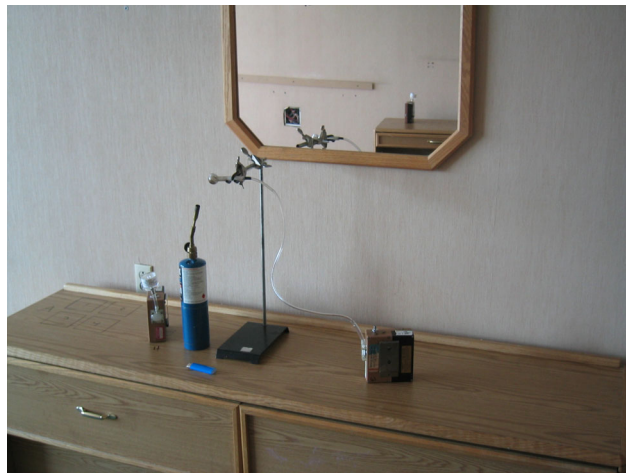
Figure 5. The sampling set-up for the “smoke” using the pipe showing the sampling setup.
